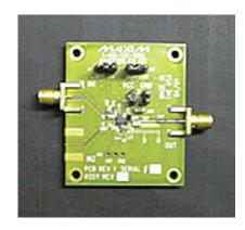
Objective: To tune linear power amplifier for Korea PCS band N-CDMA applications.
